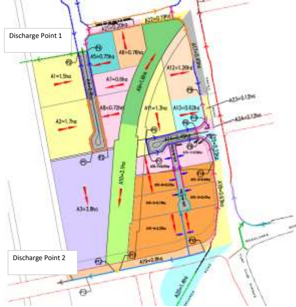
Kranji AFIP – Drainage Catchment Plan (based on permanent drain flow direction)
