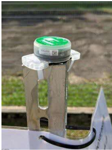
Figure 8.1 HOBO Pendant MX2202 Temperature and Light Data Logger deployed during the baseline study.
