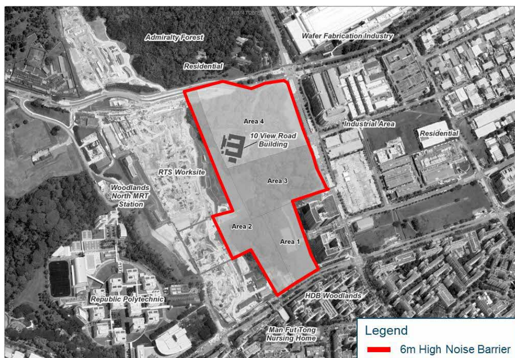
Figure 6.6 Noise Barrier Height and Extent Based on Specifications of Perimeter Noise Barriers (NEA, 2024)
