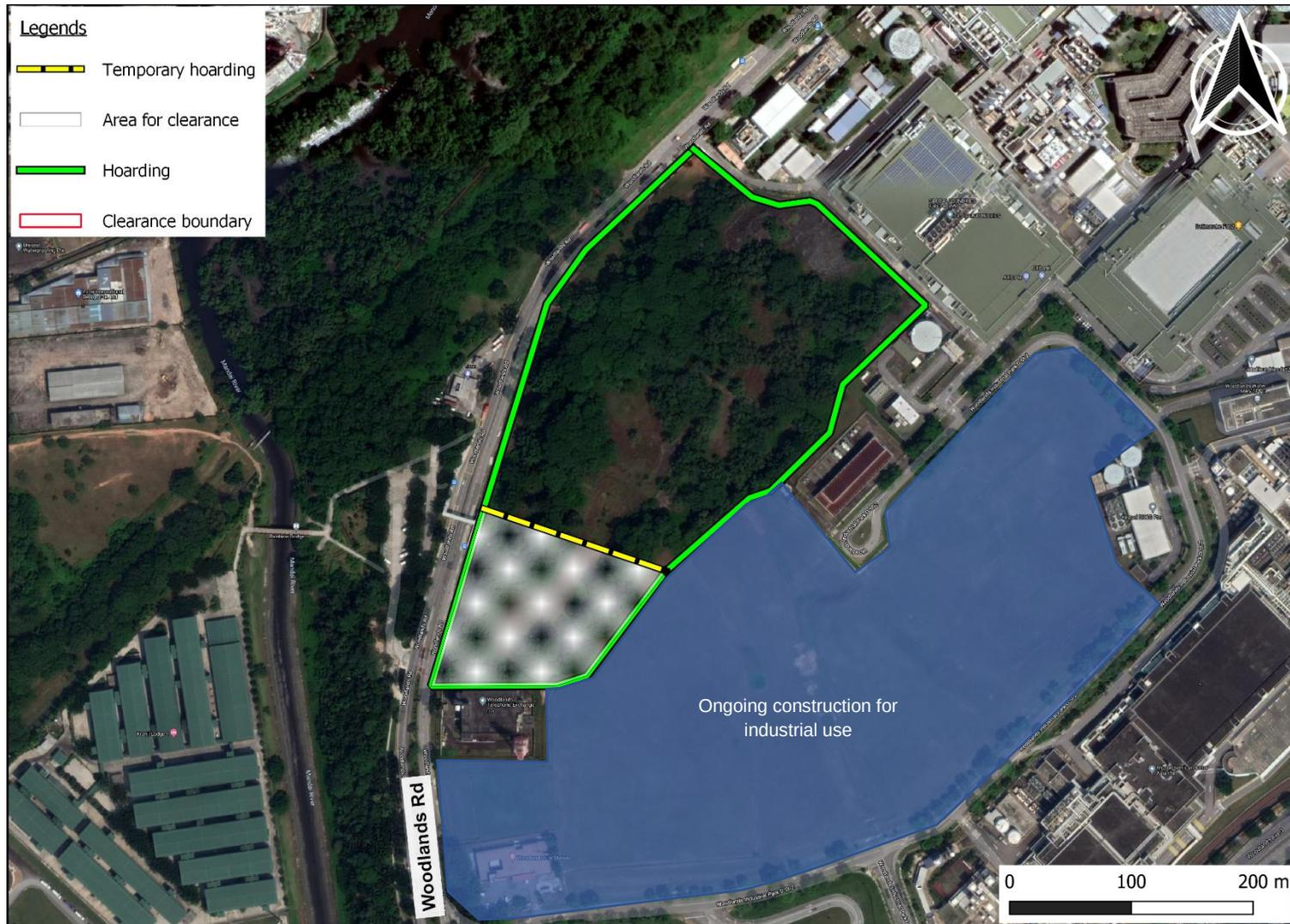
Next, hoarding shall be erected along the rest of the clearance boundary for the Phase 2 clearance.
