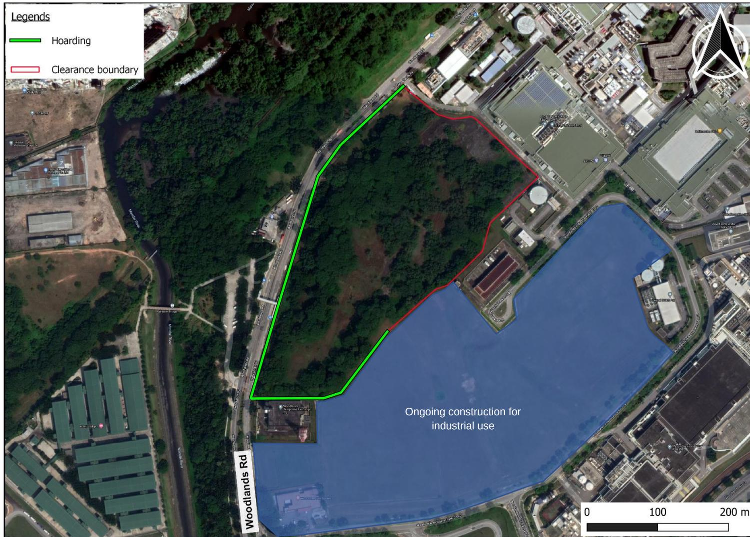
Hoarding for the Phase 1 clearance is to be erected along Woodlands Road, continuing southward before turning eastward and terminate at Phase 1 clearance boundary to prevent animals from running out into the open areas, especially Woodlands Road.
