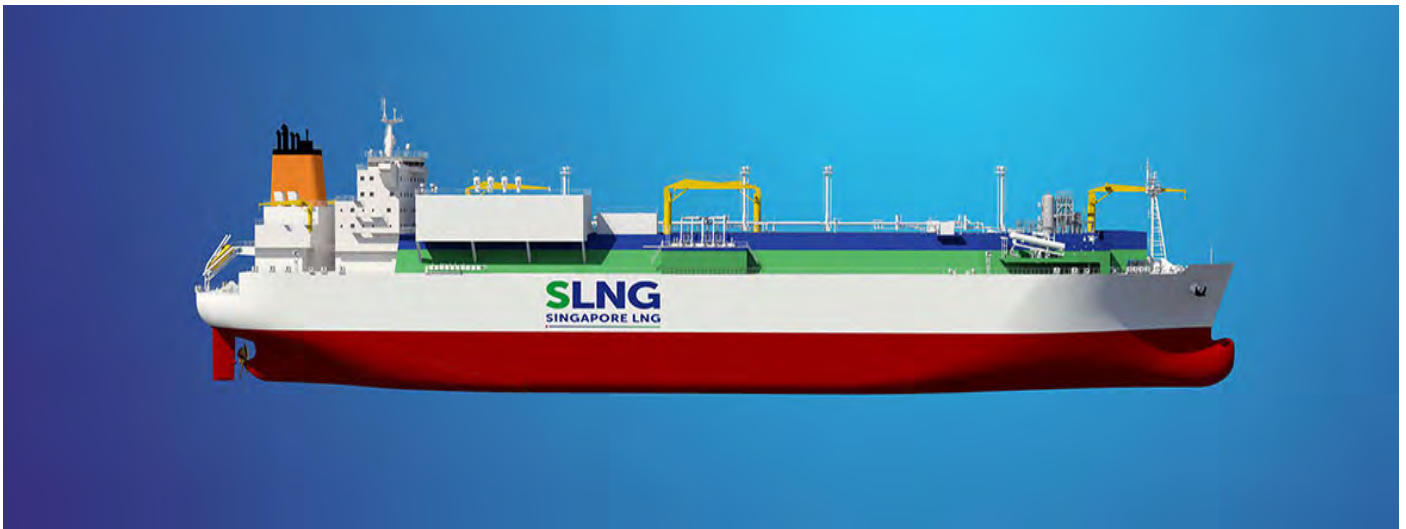
Artist Impression of the 200,000m3 FSRU which will be moored at Jurong Port
