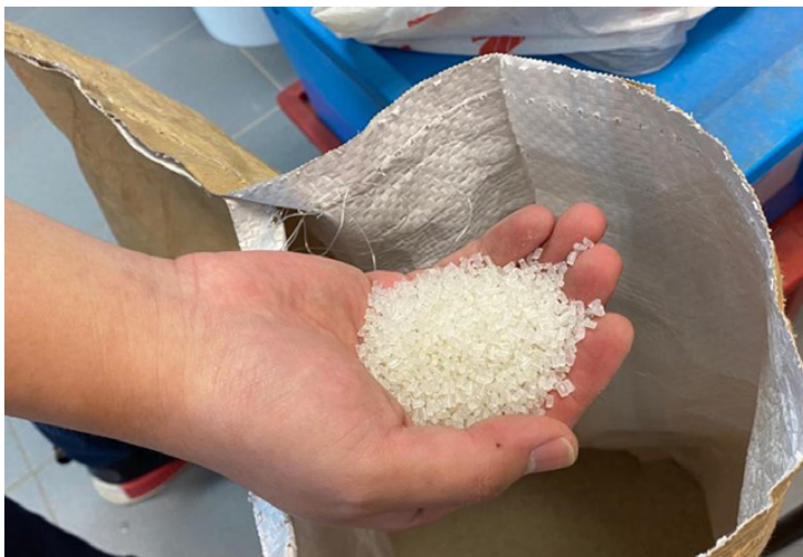
Each particle of the plastic waste (polypropylene) aggregate measures 2mm to 4mm, and is now a ready-to-use ingredient for the concrete mix.
