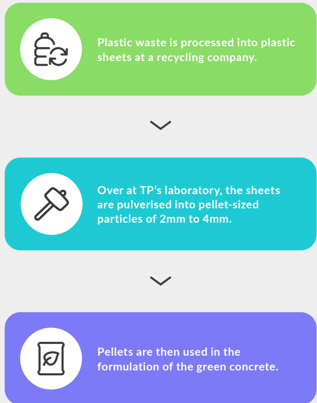
Figure 5: The process of turning plastic waste into an alternative fine aggregate
